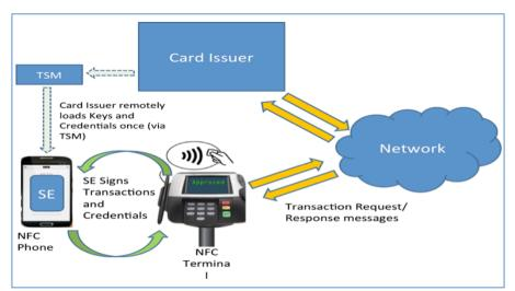
Figure 1: NFC Mobile Payments. The credentials and keys are provisioned into the SE of the smartphone. Once provisioned, the SE can sign any number of transactions (within some risk profile). The card issuer trusts the SE and accepts transactions and credentials signed by the SE.
